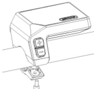
2. Then place the holding bracket on the underside of the display and tighten it into position with a M3.0\*8 screw. Torque requirement: 1.0 N.m.
